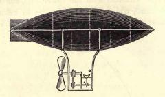
treadle mechanism, and a propeller, and the aëronaut is thus enabled to propel the balloon.
